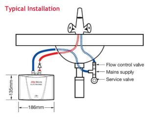
**N.B.** Zip InLine instantaneous water heating is the most efficient available, however, delivered water temperature is dependent on local incoming water temperature and supply voltage. Quoted performance assumes 12°C incoming water temperature and 230V supply.
