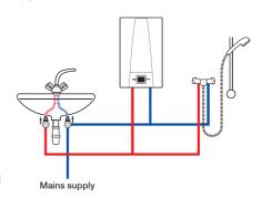
N.B. Zip Instantaneous water heating is the most energy efficient way of directly heating water electrically, however, the delivered water temperature will be dependent upon the incoming water temperature, supply voltage and selected flow rate.
